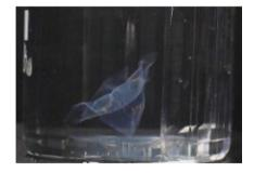
An interpenetrating hydrogel (IPH) is produced by combining a layer-by-layer polyelectrolyte membrane with agarose. The formed IPH membrane is more robust and easily manipulated and facilitates the adsorption of a stable lipid bilayer. The stable adsorption of a lipid bilayer on the IPH creates a biomimetic membrane system that is optimized for utilization in a diffusion chamber.
