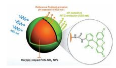
The use of core/shell structure dyedoped polymer nanoparticles in sensor films with pH and temperature sensing capabilities enables imaging of pH and temperature values with excellent spatial resolution. The new material enables referenced and temperature-compensated pH imaging with superior spatial resolution due to the use of nanosized sensor nanoparticles.
